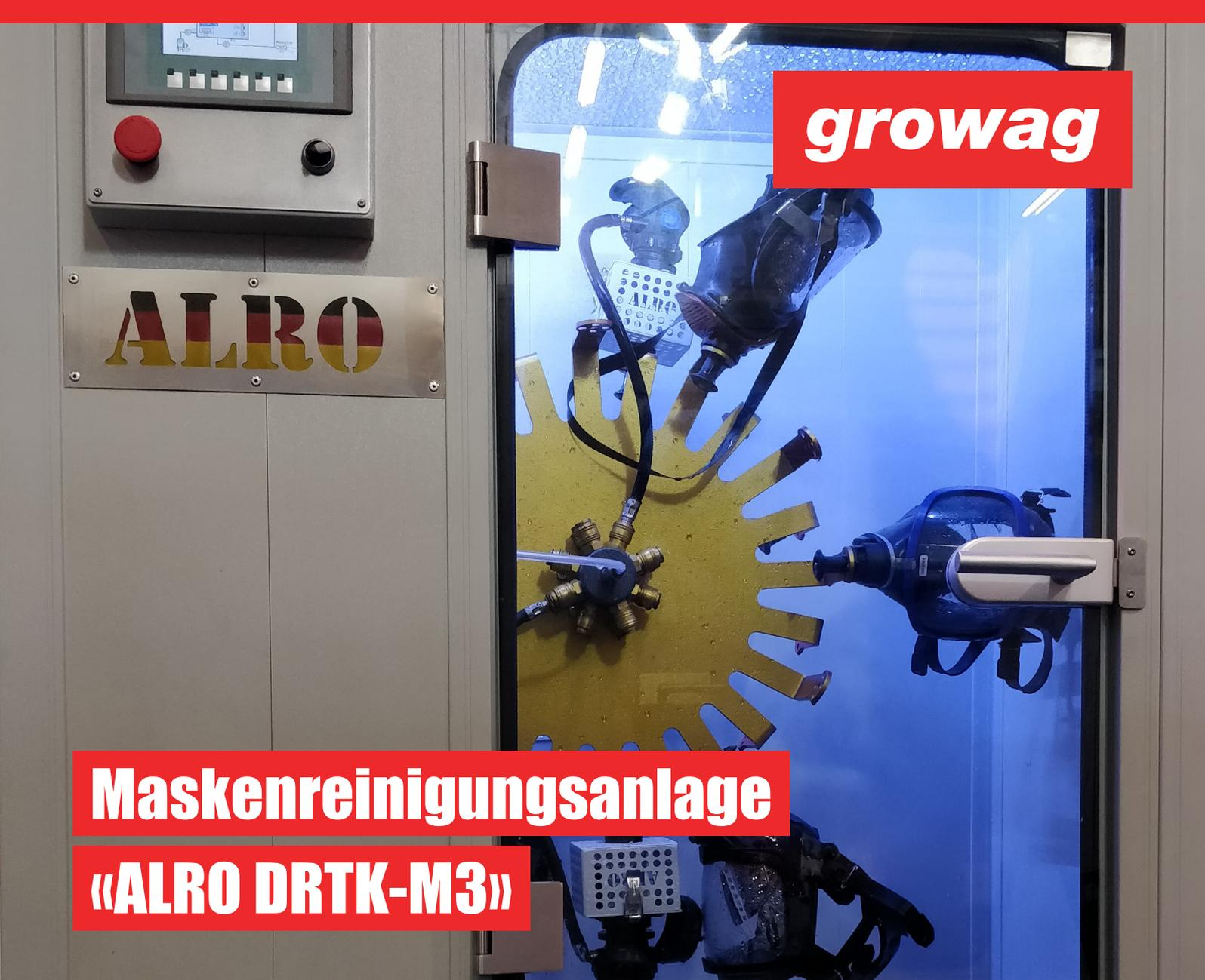
The image shows a professional mask cleaning machine. On the left, a control panel features a red emergency stop button and a digital display. The machine's door is open, revealing a central yellow gear-like structure with multiple arms. Several respirators are suspended from these arms. A blue light illuminates the interior of the machine. The brand name 'ALRO' is visible on the control panel and on the respirators. A red banner with the 'growag' logo is positioned in the top right corner.
